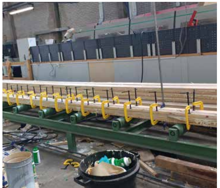
Example of a bespoke order using Accoya laminated using clamps
