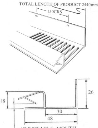
\_ ADJUSTABLE MOUTH TO FIT BOARD 4 to 12mm
