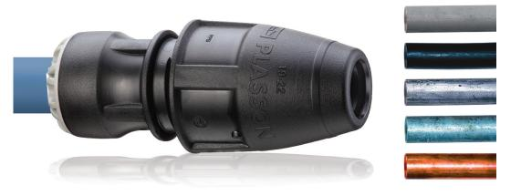
The **pushfit Universal** fitting is designed to provide a secure and reliable connection to any pipe; there are no adaptors and no loose components, just fit and forget. It requires the pipe to be slipped into fitting up to the stop, tighten the nut firmly with a wrench and that is all that is required to connect to an old pipeline!
