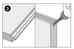
Apply Kronobuild® D4 Adhesive along the full length of both the tongue and groove profile as boards are fitted. The joints should be securely bonded when the boards are interlocked.
