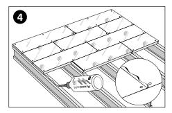
Repeat the application steps on subsequent rows of boards which should be laid in a staggered pattern. Short end joints, including perimeter edges, must fall on a secured joist or noggin. The boards must be fixed at the rate of three per board (i.e., one at each end and one in the middle). This nailing pattern gives a mechanical fixing every 1200 mm along each joist. Any excess adhesive should be left to dry then removed at the end of the build process. If in doubt consult NHBC guidelines.
