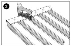
Mechanically fix the first row of boards over the joist using a fixing not less than 2 ½ times the thickness of the board. Apply Kronobuild® D4 Adhesive along the open edge profile and joists in readiness for the next board to be fitted.
