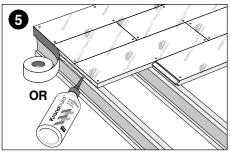
Use Kronobuild® specially formulated D4 Adhesive or Kronobuild® reinforced weather resistant tape to seal cut edges, perimeter edges, stairwells and mechanical fixing heads to reduce the risk of moisture incress
