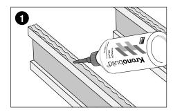
Using Kronobuild® specially formulated D4 Adhesive lay two 6mm beads to the top of the joist the first boards are to be fitted to.
