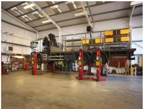
The workshop has a host of equipment, including a brake roller tester and mobile vehicle lifts, which aid the team in providing the group with an efficient maintenance service. The facility even has its own heating system which is fuelled by offcuts from the timber mill.
